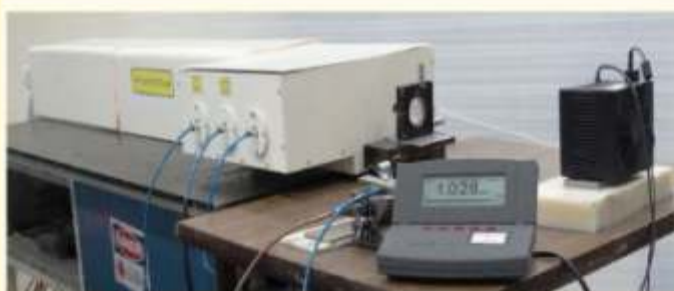
1 kW average power and 20 kW peak power Nd:YAG laser
