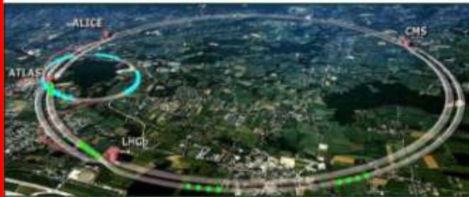
LHC, Biggest Accelerator in the world installed in 27 km circular tunnel, 100m below ground.
