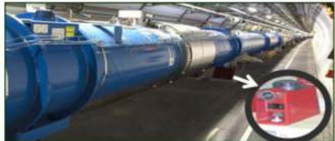
LHC machine resting on PMPS jacks supplied by RRCAT Indore
